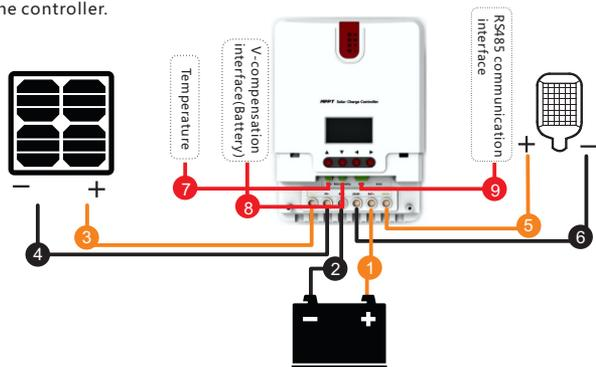
Fig. 2.3 Wiring sequence
