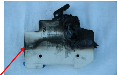
Ferraz Shawmut USM1 Touch Safe fuseholder Midnite Solar part number - MNTS
