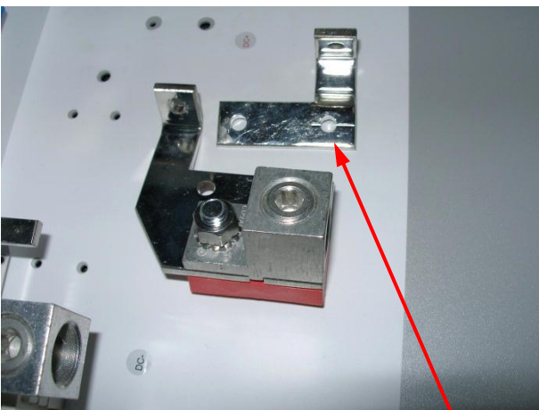
Remove two bolts holding small busbar. Remove small busbar from PV positive lug
