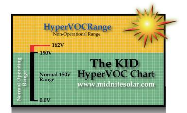
**Above:** HyperVOC voltage limits above normal operating voltage.
