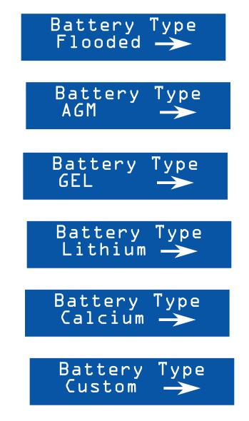
Stop on the correct battery type and then hit the right arrow key. It then takes you to the absorb voltage screen.
