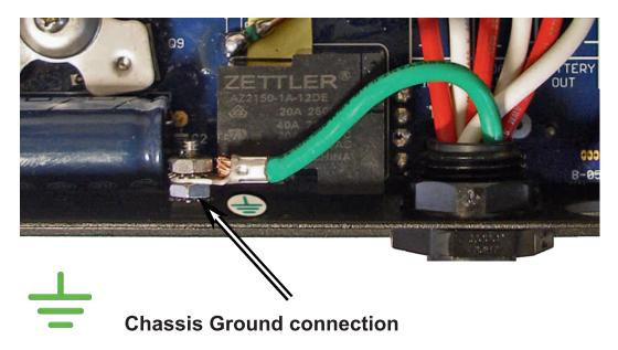
The screw, nut, and terminal for grounding the chassis are included on all models. The chassis ground (equipment ground) is required in an NEC compliant system. The chassis of The KID is isolated from all internal KID circuitry. Wall mount versions have a short wire pre-installed in this location. It can be found in the wiring area of the wall mount.
