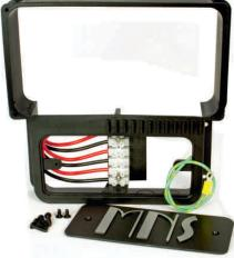
Make the wire connections to the terminal block inside The KID, replace the back plate and then assemble The KID to the wall mount adapter. Use the  $#10 \times \frac{3}{4}$ " Plastite screws provided to secure The KID to the wall mount adapter.
