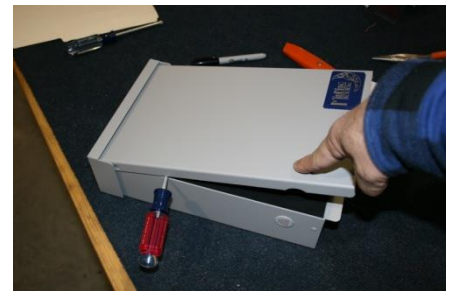
Remove top cover prior to removing the deadfront on Type 3R units.
