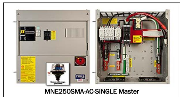
The backed up critical loads panel always has 120/240vac available. 60amps is available on leg 1 and 30amps on leg 2 in the critical loads panel. Comes standard with one MNSPD-300 (surge protection device).
